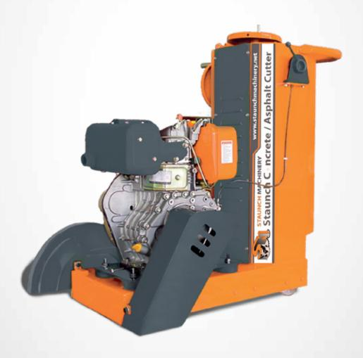
The Concrete / Asphalt Cutter is powered by a Robin EY40 engine, or a Honda GX340-11HP engine, or a Staunch 11HP Diesel engine. The cutter is equipped with a built-in 30LT steel water tank and a steel shaft Plummer with a double bearing. The blade on the cutter can have a diameter of 40cm that can cut through asphalt or concrete up to 15cm in depth.
